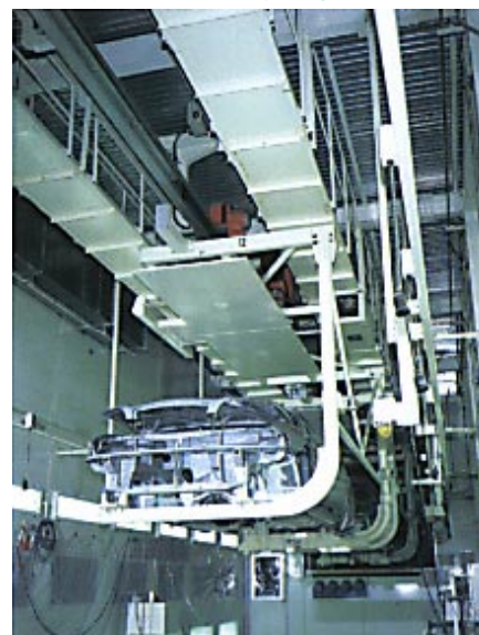
Monorail system for automobile painting
