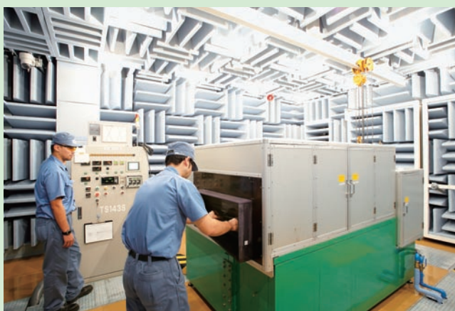
Testing in anechoic engine bench room
