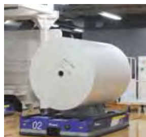
AGV roll paper feeding system
