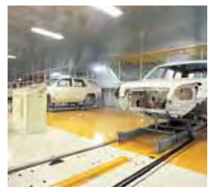
Conveyance system for automobile painting lines
