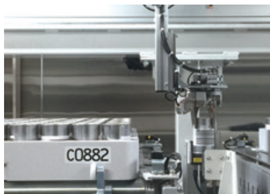
Tsubaki Labo Stocker employed by NIAS Genebank for permanent storage of seeds from around the world under low-temperature, low-humidity conditions
