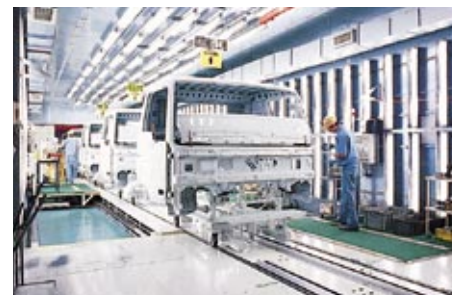
New Traverser System
