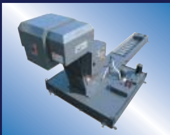
Scrap metal conveyance and coolant system
