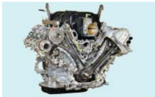
Timing chain drive system applied to V8 engine
