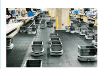
T-Carry System, a handling and sorting system using small AGVs (2020)
