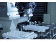
LaboStocker, an automated cryogenic storage system for regenerative medicine and new drug discovery (2011)
