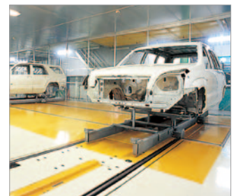
Conveyance system for automobile painting lines
