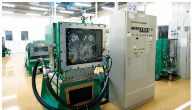
Timing chain drive system test simulator at the Auto Engineering Lab
