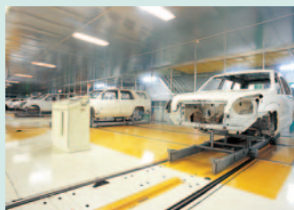
Conveyance system for automobile manufacturing lines
