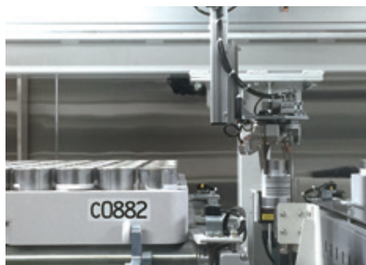
Tsubaki Labo Stocker employed by NIAS Genebank for permanent storage of seeds from around the world under low-temperature, low-humidity conditions
