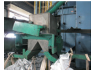
Magnetic separator used for separating sand from other particles
