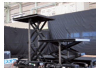
Lift system synchronously operating four Zip Chain Lifters for supporting concert performers (Shimizu Octo factory)
