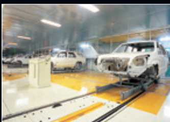
Conveyance system for automobile manufacturing lines
